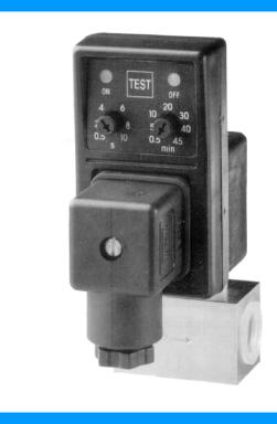
This is designed to provide a solution for the automatic draining of filter bowls., Separators, dryers, receivers, drip legs and other compressed air system components where condensate and contaminants collect. The draining interval and discharge time can be adjusted according to all requirements.
